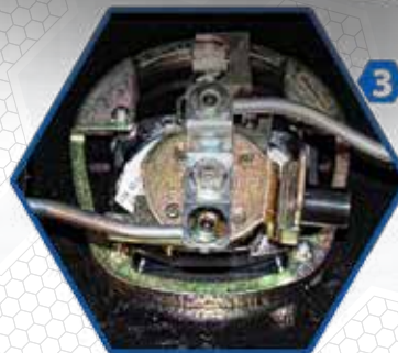
DUAL LOCKING CAM ACTION LOCKS
